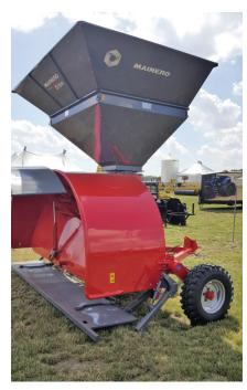
The Mainero 2241 now features a hydraulic bottom tray, which allows for easy and simple bag loading!
